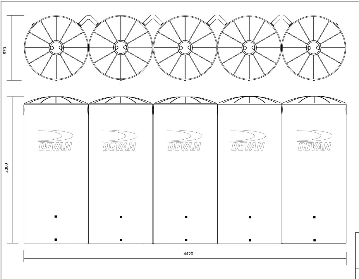
NOTE: Tanks are delivered as individual 1000L pods, assembly required onsite
